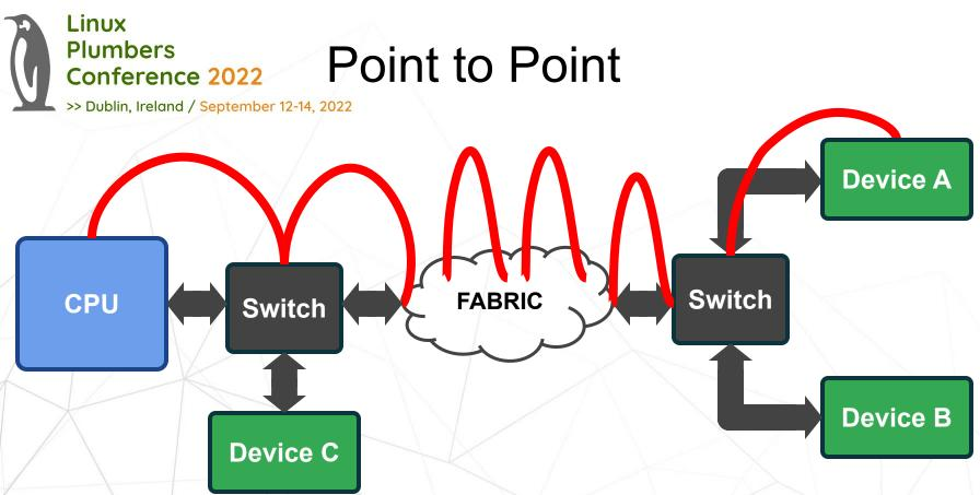
Integrity & Encryption between each point along a path ⇒ Have to trust each point in a path (each has access to plaintext)
