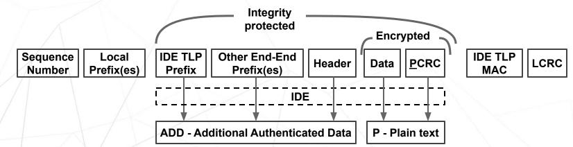
[Encryption key] + [some counter / salt (receiver side can predict)] ⇒ Encrypt data payload (& CRC)
