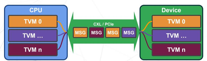
Protect Trusted Virtual Machine (TVM) End to End ⇒ Identify TVM Traffic
