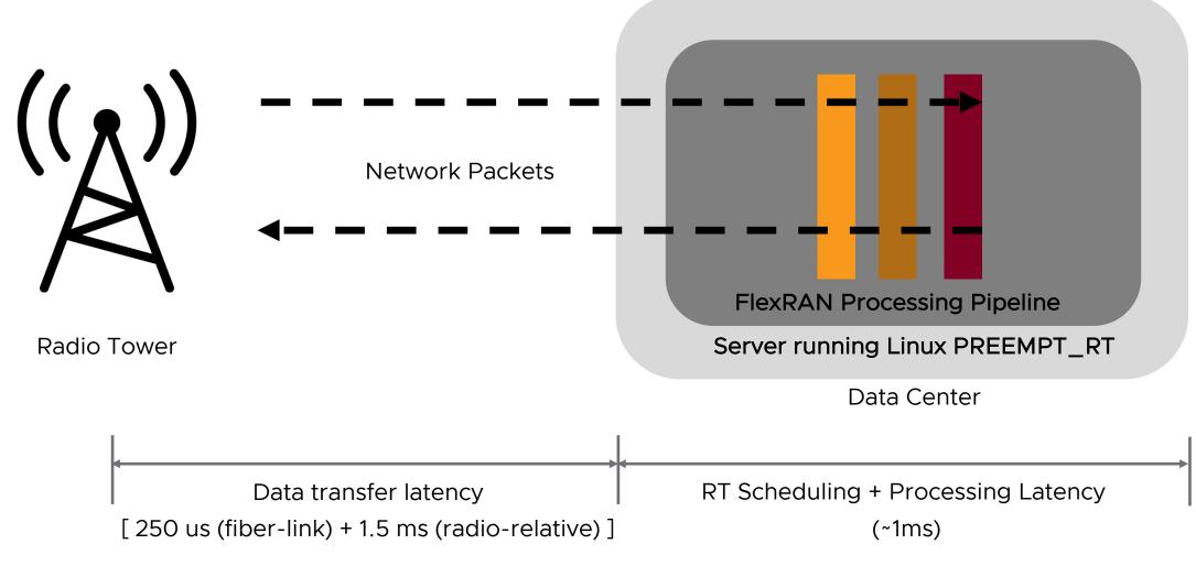
Fixed total latency budget for packet Tx + processing + ack (< 3ms)
